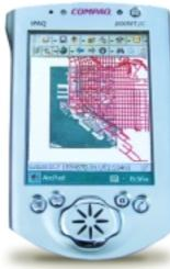
ArcPad software by ESRI is a data collection system and a mobile GIS. It supports a multi-layer environment with industry-standard vector map and raster image display that includes aerial photographs and satellite imagery. Other primary
